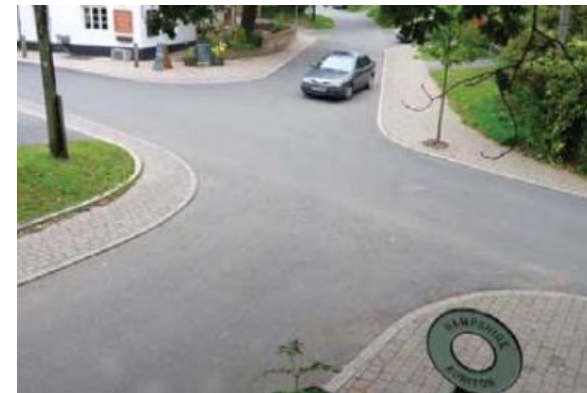
Footway build-out providing a sense of arrive and space for planting, narrowing carriageway by creating pinch point and horizontal deflection
