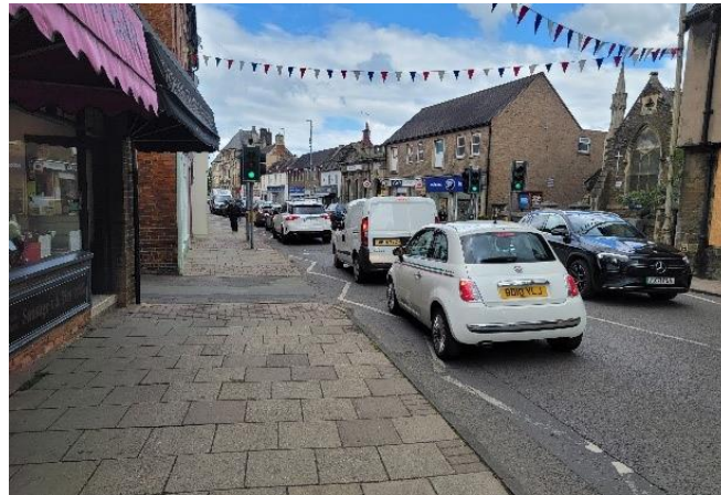
Very wide junctions such as B640/ Northgate/ Station Rd can encourage faster vehicle speeds and discourage pedestrian movement in the town centre.
