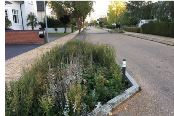
Footway build-out providing a sense of arrive and space for planting, narrowing carriageway by creating pinch point and horizontal deflection
